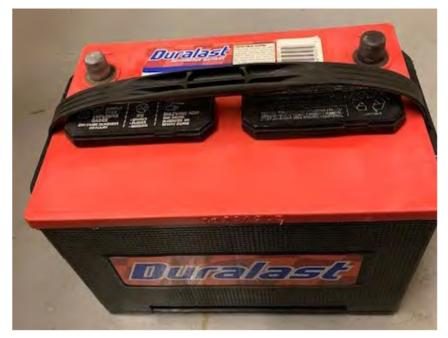
The battery's function is to provide current to start the engine. Once the engine is running, the current required to keep everything like the ignition system, bilge pump, lights and other components operating, as well as replenishing the current used to start the engine comes from the charging system, provided it has adequate charging capability. In theory, once the boat has started, current is provided by the charging system, and you no longer need the battery until the engine is stopped.
