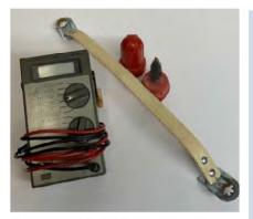
A DVOM (Digital Volt-Ohm Meter) is indispensable for trouble shooting an electrical problem. Perhaps the handiest item is a battery carrying strap which attaches to the terminals and allows the battery to be safely lowered into close fitting boxes and surroundings as well as carried without having to cradle it and get acid on your clothes. The battery terminal brush allows the terminals and clamps to be properly cleaned.
