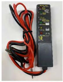
One of the best tools for somebody who just needs a quick analysis. It gives a quick reading of the charging system as well as the battery condition.
