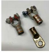
These are the best terminals and clamps to use. Have them crimped on, then fill the crimp with solder to ensure a conductive connection as well as a good mechanical connection. Heavy duty truck dealers can supply the proper cables and do the crimping.
