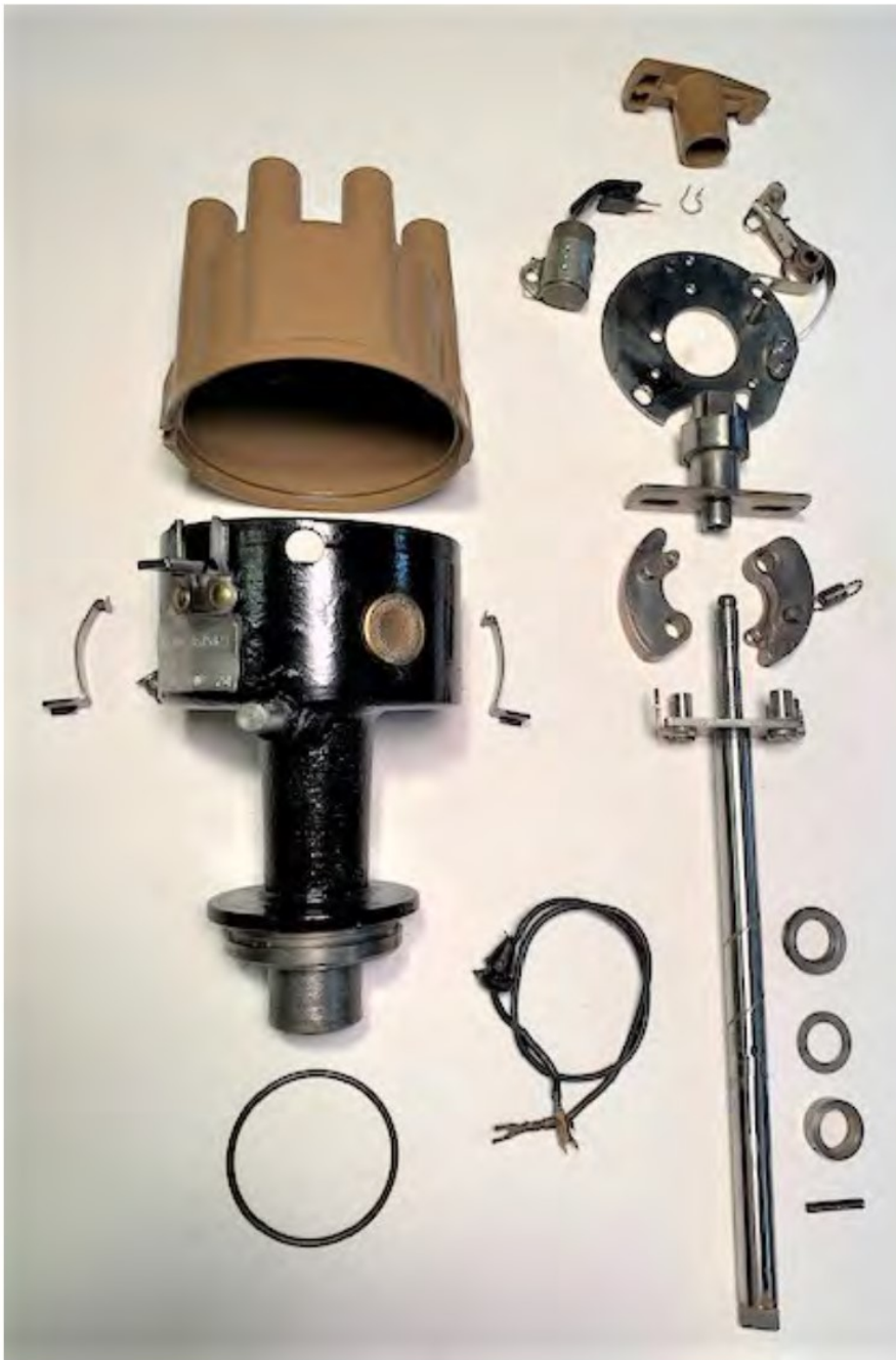
Fig. 6 – The components for a typical marine distributor with mechanical advance only. Note the special bronze USCG approved flame arrestor screen located in the non-vented housing required for all marine distributors.
