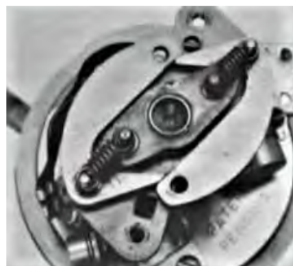
Fig.4 – Showing the mechanical advance weights used to advance the distributor cam as RPM increases.
