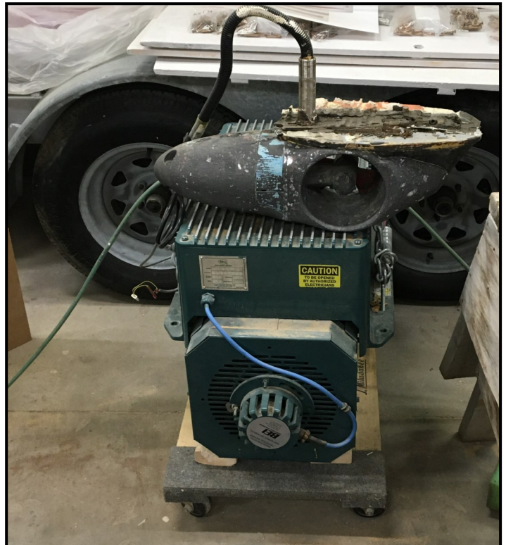
Bow thruster resting on top of Elco power plant.
