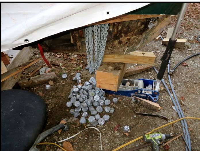
Lead and chain ballast removed.
